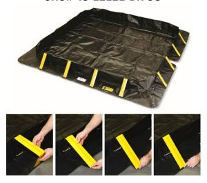
Stinger Snap-Up berms are ENPAC's most popular and intuitive containment berm. Available in a wide variety of sizes, the triangular stays create a sturdy sidewall and are welded in place, leaving no loose part that can be lost. Setup is a snap: simply slide the bottom portion of the stay into the appropriate skirt pocket, and your chemicals are fully contained. The sidewall can easily be laid flat to be driven over by vehicles and other equipment.
